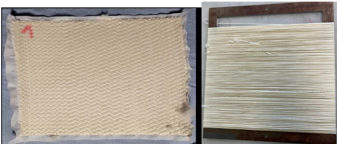
Fig. 3: Embroidered preform (left), wound preform (right)
