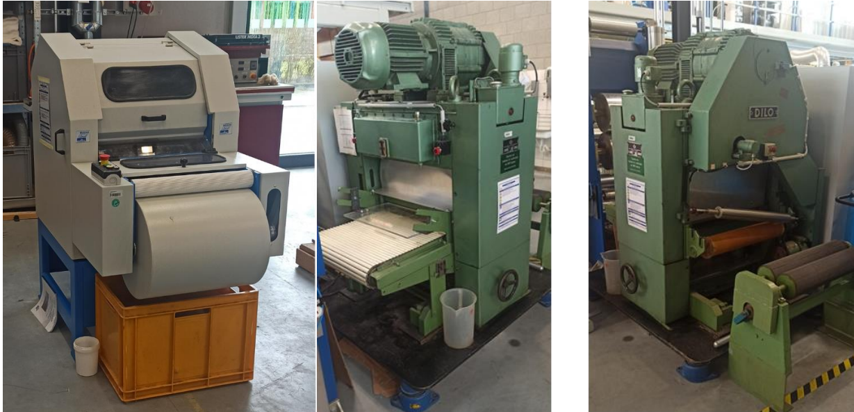
Fig. 2: Carding machine (left), needle punching machine (center and right)
